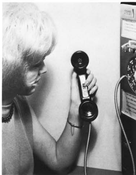
The volume-control handset is demonstrated by Mrs. Peggy Ballard of the Indianapolis Laboratory. A switch in the handle can be used by customers with impaired hearing to amplify sound coming from the receiver. The spring-loaded slide switch returns automatically to a normal setting so the handset is always ready for normal use.
