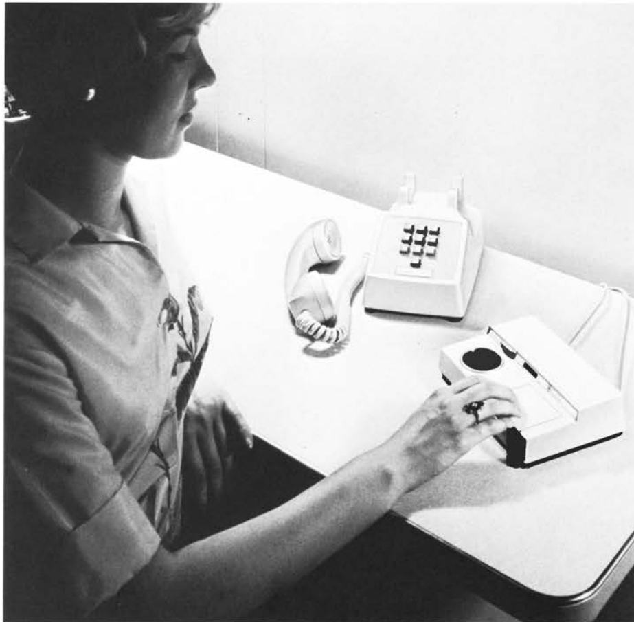
The new Code-Com set for the deaf is demonstrated by Miss Janine Sliwa of the Indianapolis Laboratory. The set, connected to a conventional telephone, will allow a deaf person to "see" phone messages in coded flashes of light or "feel" them in the vibrations of a finger pad. Light flashes come from a recess (black rectangle) in the center of the raised portion of the set. The circular vibrating pad is on the left. The sending key, used like a telegraph key, is on the right.
