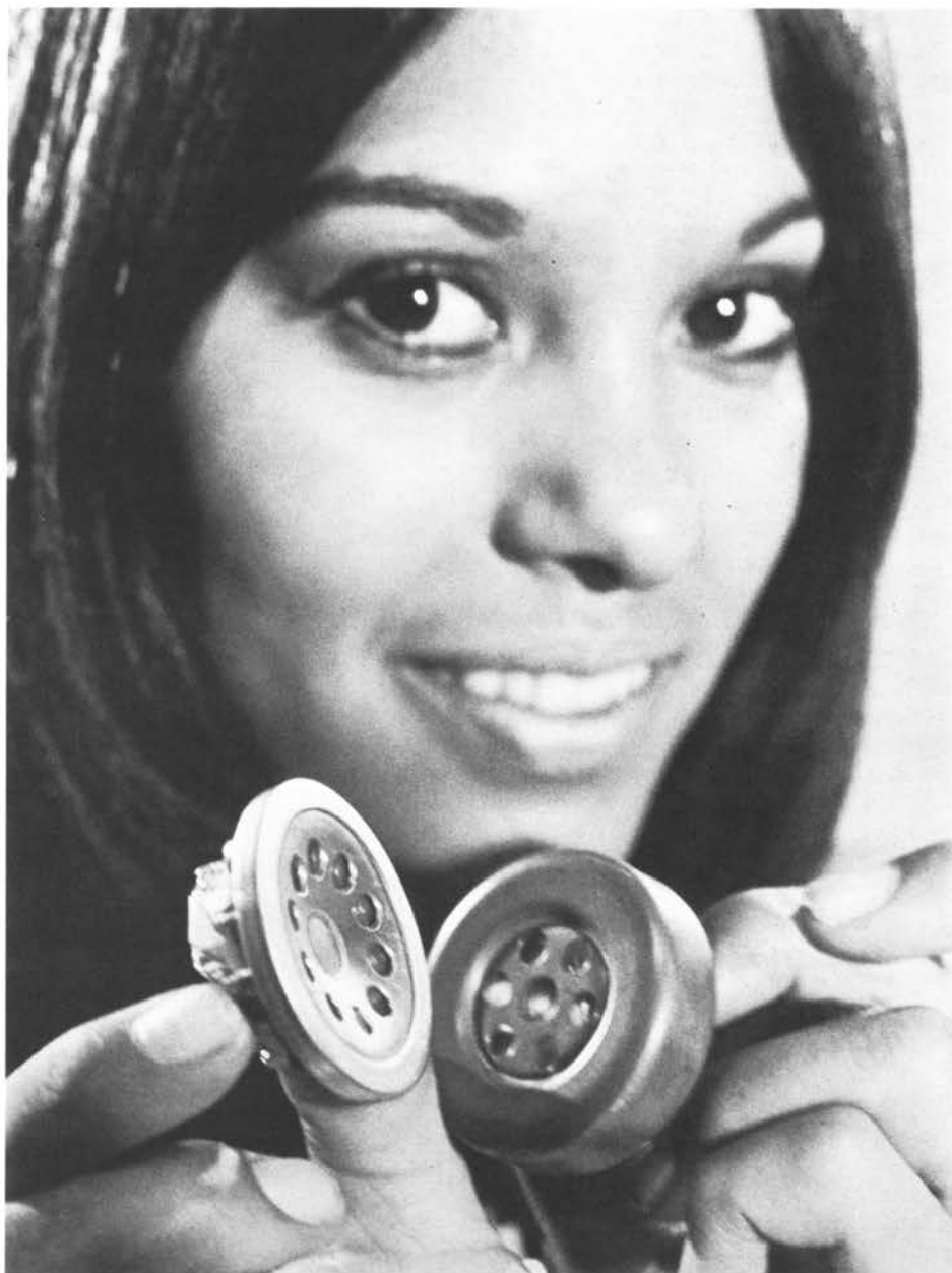
Bell Labs' Diane Johnathan holds a standard telephone receiver (right), and a smaller, improved unit (left) which will eventually reap a savings of more than two hundred tons of strategic raw materials per year. The estimated savings in materials is based on an anticipated annual production rate of 10 million units. The new receiver will eventually be used in most Bell System telephone sets.
