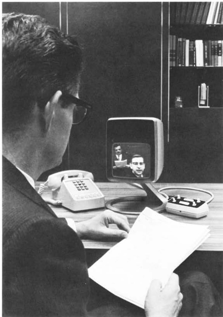
1968 The Bell System's PICTUREPHONE "see-while-you-talk" set has been redesigned to incorporate additional features as a result of the extensive trials. The improved "Mod II" set shown here will itself be the subject of further trials during the continuing evolution of PICTUREPHONE service.
