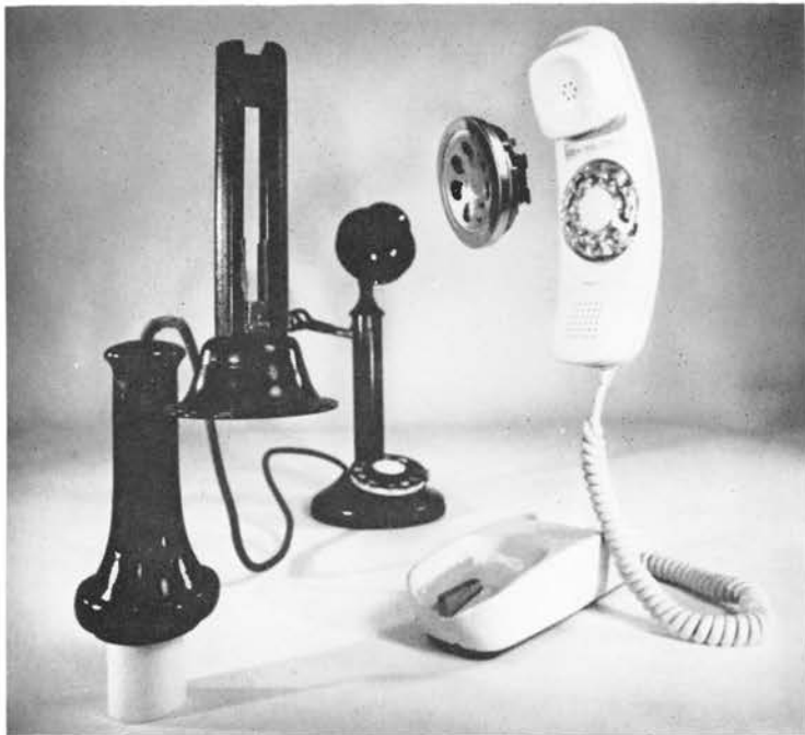
The dumbbell shape of the 1905 receiver was dictated by the long bar magnet required to produce an adequate signal. Technological advances have resulted in the LB1 receiver for the TRIMLINE handset. This unit is only \frac{1}{18} as heavy and \frac{1}{8} as high as the 1905 model.
