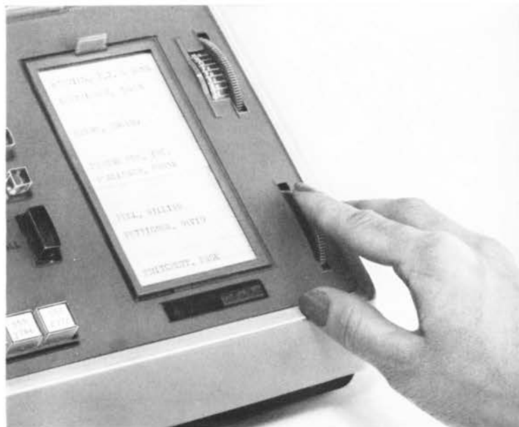
Two finger wheels are used to look up numbers in the CALL-A-MATIC phone's directory. Setting the upper wheel causes a motor to run the directory tape to one of 50 positions, 10 spaces apart in the directory. The lower wheel is geared to the drums that carry the directory tape; it moves the tape manually for selecting the individual space desired. Both wheels are disabled while a customer is trying to record a number in the repertory or place a call.
