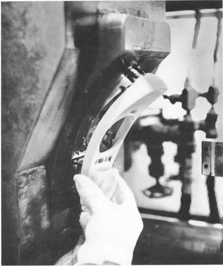
This injection molding machine is one of many at the Indianapolis Laboratory, which will produce about one and a half million TRIMLINE telephones this year.
