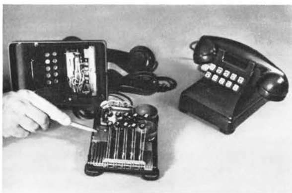
Telephones used in the 1948 trials of push-button calling. Pencil shows transducer that picks up tones from plucked reeds (fixed to the base behind the key levers). Note arrangement of buttons.
