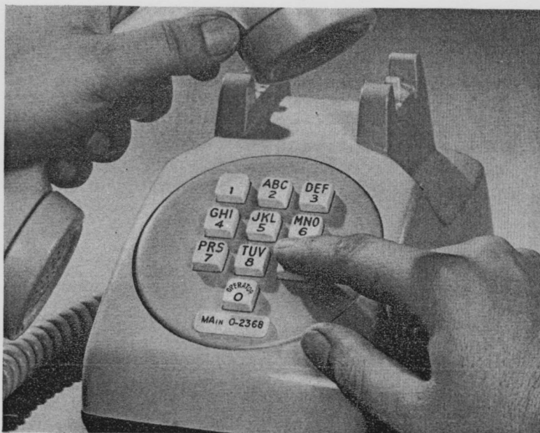
Laboratories experimental push-button set (also see cover). Push-button unit here includes changes made subsequent to trial model.
