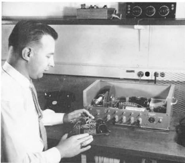
Fig. 5 — J. Kocan observes the operation of an experimental photo-electric signal generator that supplies the complex tone ringer signal voltages for the development laboratory.
