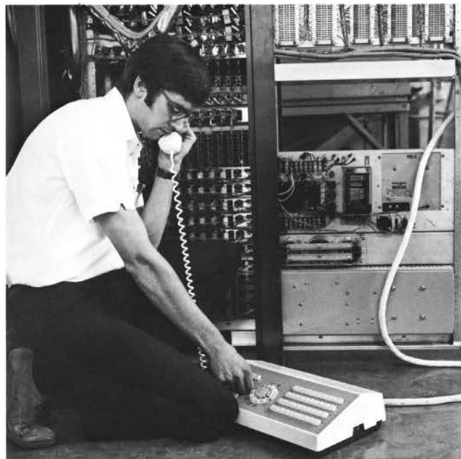
The switching cabinet of the 558A PBX has sliding equipment racks for easy access during installation and maintenance, as demonstrated here by installer Paul Jaeger of the New York Telephone Company. Even though the cabinet may be installed in a remote area of the customer's premises, plug-in connectors enable Jaeger to bring the console to the circuits for testing.
