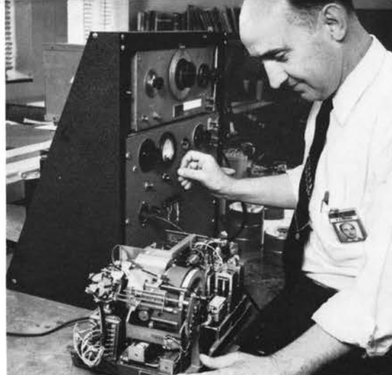
Fig. 3 — W. R. Goehner using a 2A answering set to test "magnetic rubber" recording bands.
