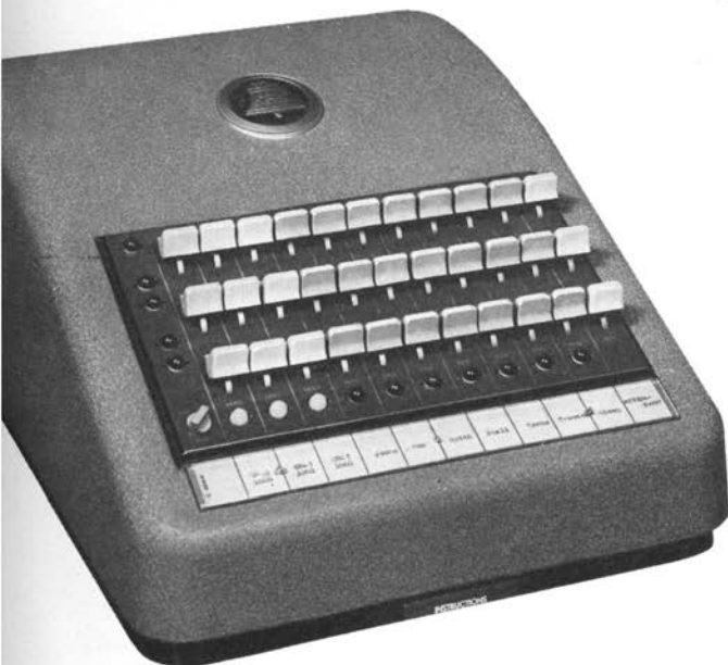
Fig. 1—The 507A PBX has capacity for three central office trunks and seven extension lines.
