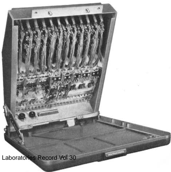
Fig. 3—The chassis is hinged, and may be lifted to expose the wiring.
