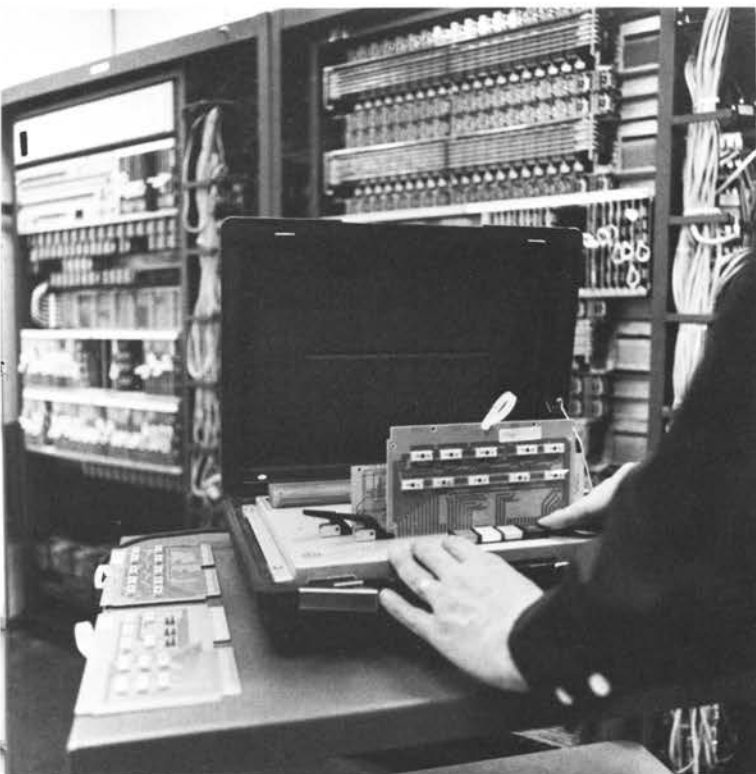
Testing circuit packs in the field. Craftspeople can check whether circuit packs are good or bad by plugging them into this portable test set and pressing the "test" button. A lighted lamp indicates whether the circuit pack "passes" or "fails."
