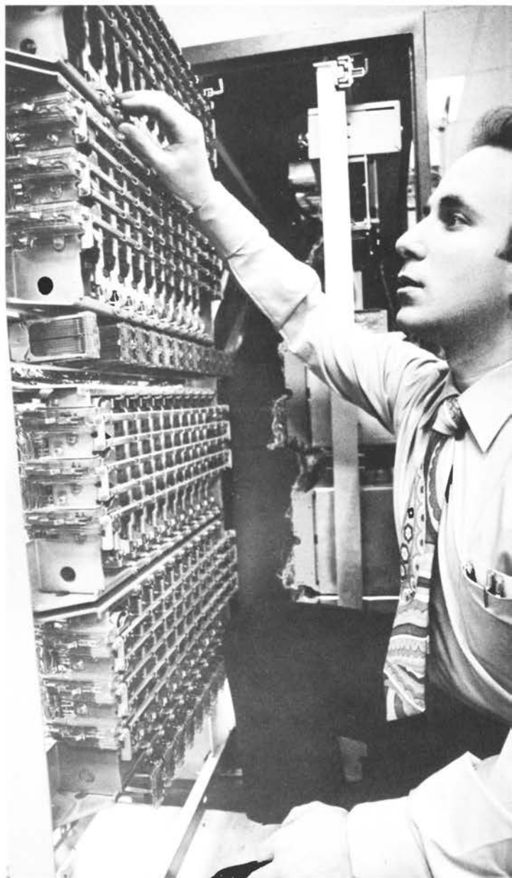
Raymond Dellecker and David Weiner, above, test a prototype model of the 805A at Bell Labs' Denver location. One of the slides, holding the power supply and electronic circuitry, is shown extended from the cabinet. The other slide is visible through the space left by the extended slide. In the right-hand photo, Weiner (formerly of Bell Labs' Denver facility, now with AT&T), examines the crossbar switching units. The crossbar is the same as those used in No. 5 crossbar central offices.
