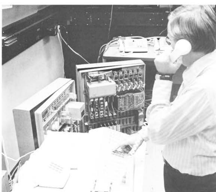
John Evans of Bell Labs tests a 4A call distributing system from the supervisor's console (foreground) at a laboratory in Holmdel, N. J. The equipment is compact and easy to transport.
