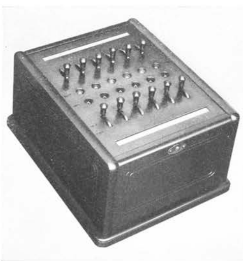
Fig. 1—A six-line double-sided keybox for Multiple Line Key Equipment, showing the single assembling screw
