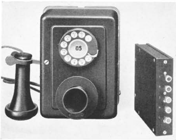
Fig. 2—A separate key is arranged for use with desk stands or wall sets
