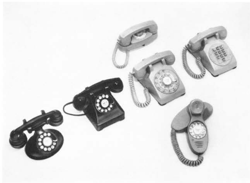
This group picture shows recent trends in handset design. Two earlier designs, in black, are shown at left. Group at right consists of 500-type set with dial, experimental unit with push buttons, Princess Set, top, and new experimental Dial-In-Handset. The Dial-In-Handset is the first radical departure in handset design.
