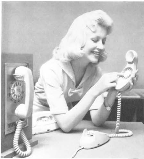
Miss Barbara Weiss of the Laboratories tries the new Dial-In-Handset. At her elbow is the new Princess Set, and at the left is an experimental panel model mounted with its base flush with wall.
