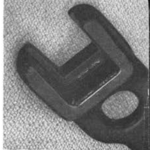
Fig. 2—One end of the wrench showing two sizes of openings and the elliptical hole.
