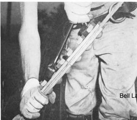
Fig. 3 (left)—Tapered faces of "B" lineman's wrench set wrench shank at an angle to the work so that the shank and the workman's hand clear obstructions as the wrench is turned. Fig. 4 (right)—With the end of the steel pole step in the elliptical hole in the shank, the wrench becomes a lever either for turning the step into proper position or for unscrewing it from the pole.
