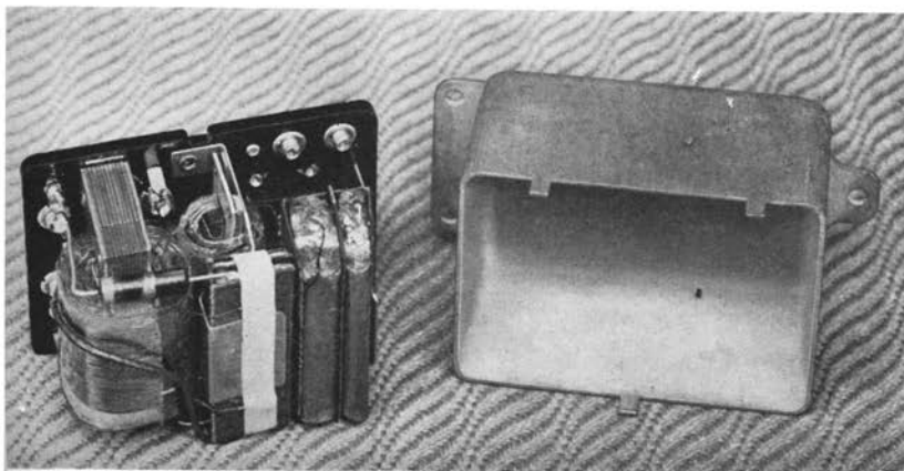
Fig. 4—Elements of the seven circuit components of the 425A network.
