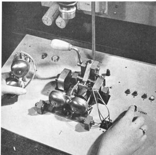
Fig. 2—C-type ringer in position for adjustment. Lights at right signal success or failure.
