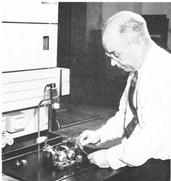
Fig. 1—A. F. Conk connects ringer to automatic adjusting set.
