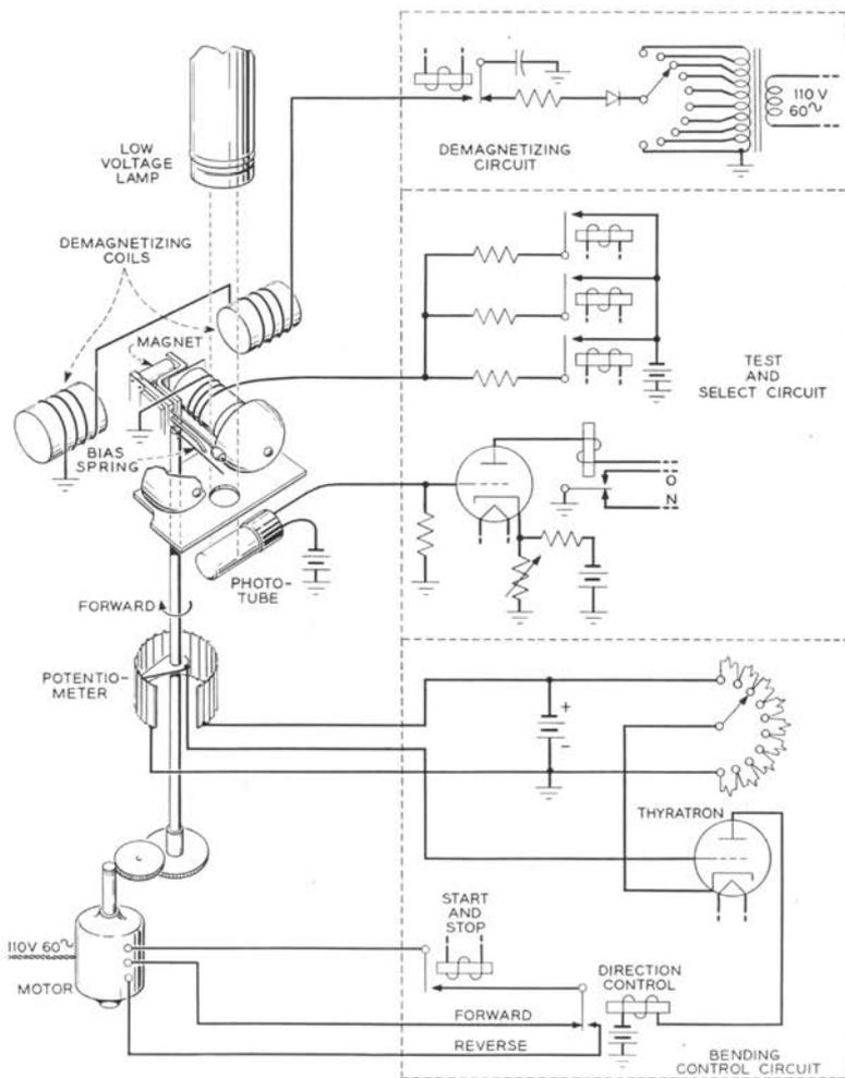
Fig. 4—Diagram showing operation of ringer adjuster.
