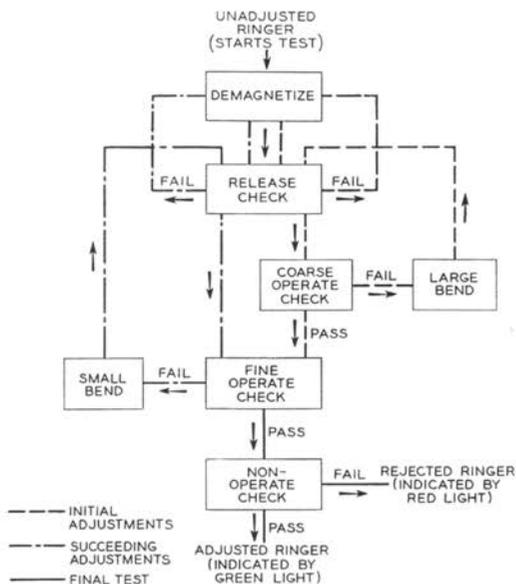
Fig. 5—Flow chart of ringer adjustment process.
