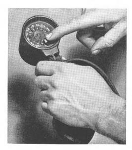
N DIAL-telephone areas installers have been using a dial-type handset with a metal handle. A new piece of equipment has now been developed which has several advantages. It is lighter, more compact and has improved transmission which arises from its utilization of the same units for transmitter and receiver as the F-type station handset. It has a rubber handle which renders it more resistant to damage from impact and handling than its predecessor.
