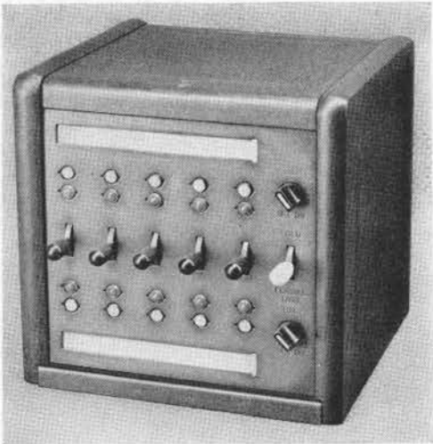
Fig. 2—The keys and lamps are arranged in ten-line units, and each unit has a common holding key
