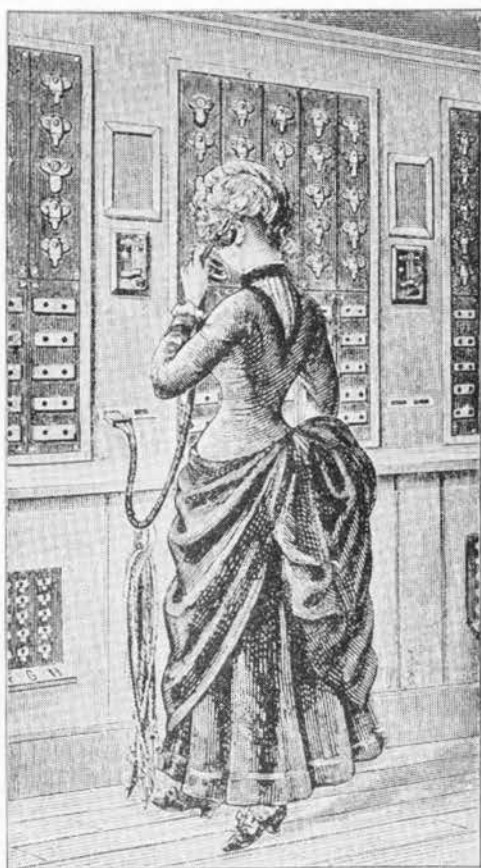
Fig. 4—Brown took his early handset to France, where it was used in the early Paris exchanges
