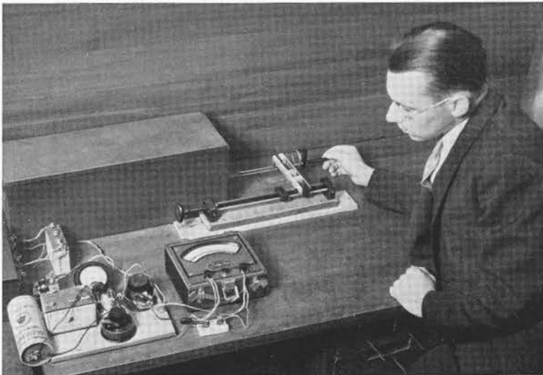
Set-up for measuring the "q" of circuits tuned for wavelengths in the neighborhood of 60 centimeters. W. E. Kirkpatrick of the Research Department is adjusting the microscopic condenser of the tuned circuit
