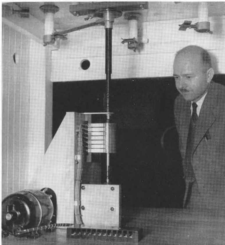
A final inspection of an antenna switch before it is shipped to Miami. The switch, housed outdoors and remotely controlled from the transmitter room, will connect a two-wire line from a short-wave transmitter to the lines to any one of six directive antennas. Contacts for one side of the lines can be seen fastened to the ceiling. Those to the other side are in the compartment above. It will be used in radiotelephone links between the United States and points bordering the Caribbean Sea. The inspection is being made on the Laboratories' shipping platform by J. L. Mathison, of the Radio Research group.
