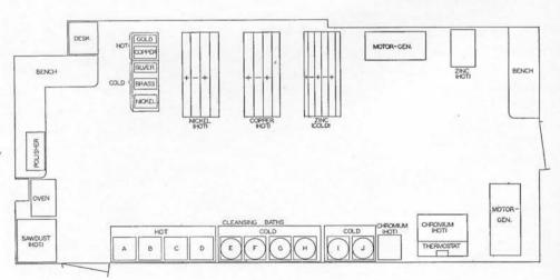
Fig. 4—The plating room is located in section 3-B. The cleansing baths are: A—clean water; B—soap solution; C—preliminary wash water; D—alkaline electrolytic cleaner; E—bright acid dip; F and G—hydrochloric acid pickels for (F) steels and (G) brasses; I—cyanide dip; H and J—clean running water
