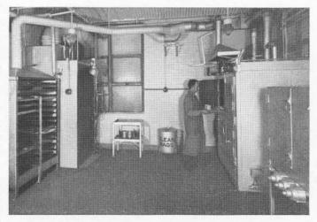
Fig. 3—The japan room. Left to right: drying rack, small spray booth, baking oven (into which Charles Stone is placing equipment he has just sprayed), and crystalizing oven.
