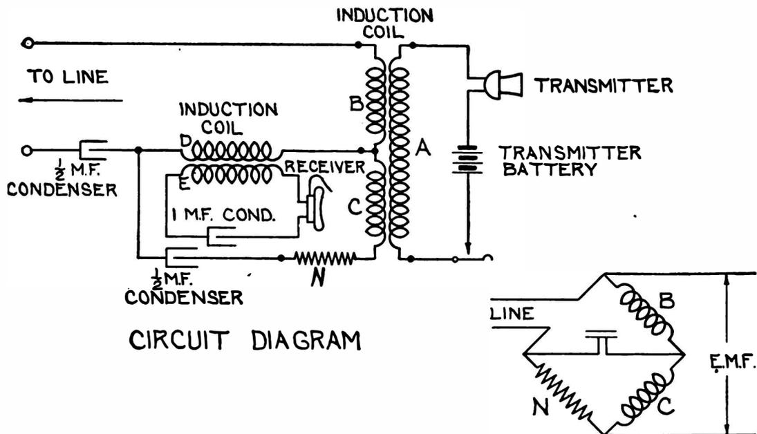
Fig. 15—Dispatcher's Set for Non-Loaded Open Wire Metallic Lines and Loaded Cable Circuits
