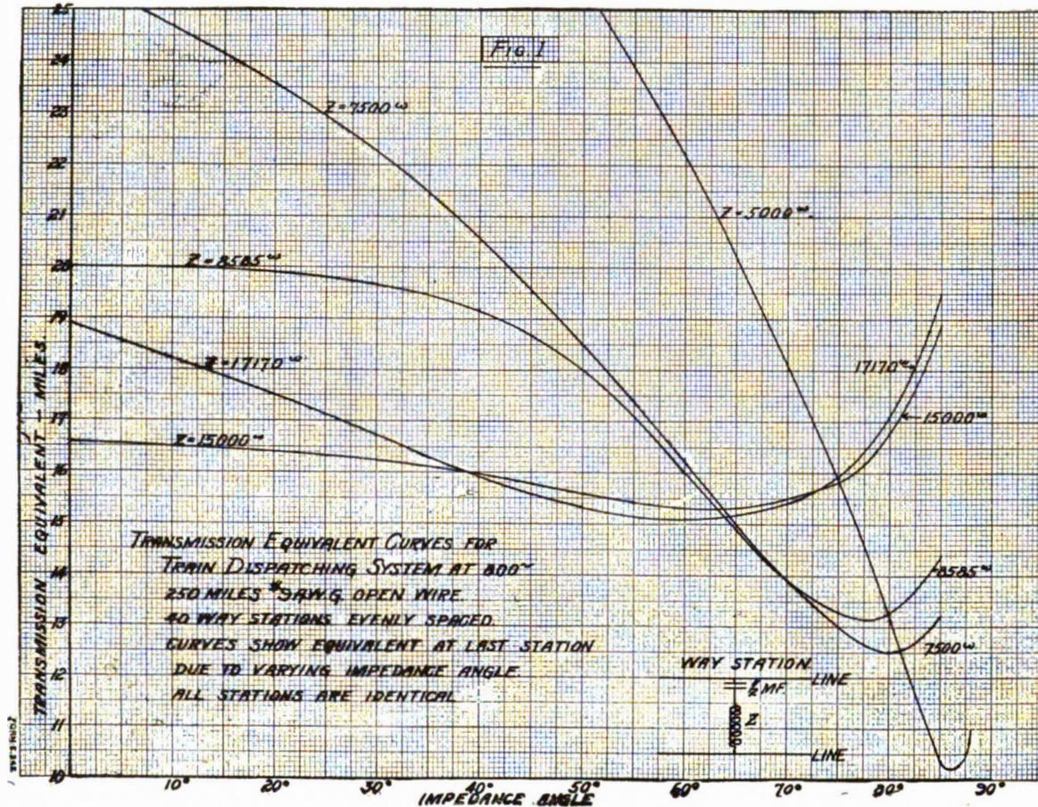
Fig. 1—Transmission Equivalent Curves for Train Dispatching
