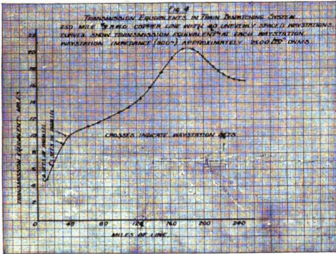
Fig. 4—Effect of Spacing Stations Irregularly
