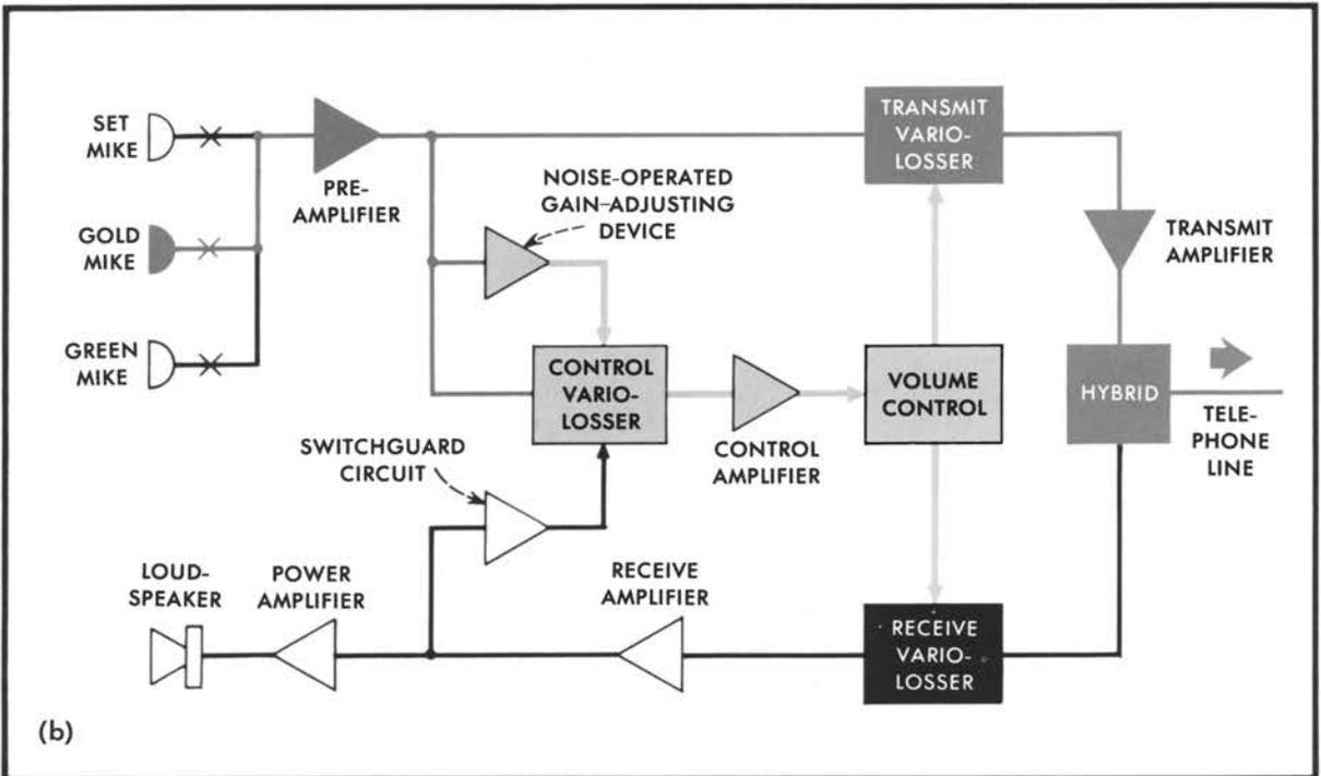
When the PCT is in the receive mode, upper diagram (a), incoming speech is tapped off by the switchguard circuit. The control variolossor and control amplifier then increase the loss in the transmit variolossor, almost cutting off the trans-
