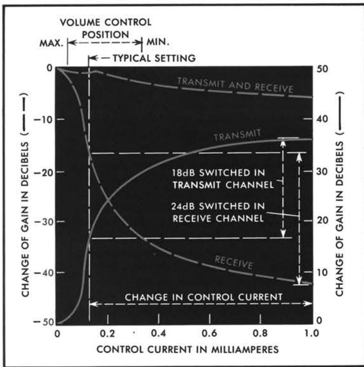
The PCT's transmit and receive variolossers operate together—when one increases its loss, the other reduces its loss. The control current for each variolossers ranges between 1.0 milliamperes and a lower current, determined by the setting of the volume control. In the receive mode, the current is set by the volume control. When the user speaks, the current increases, raising the loss in the receive channel and decreasing loss in the transmit channel.
