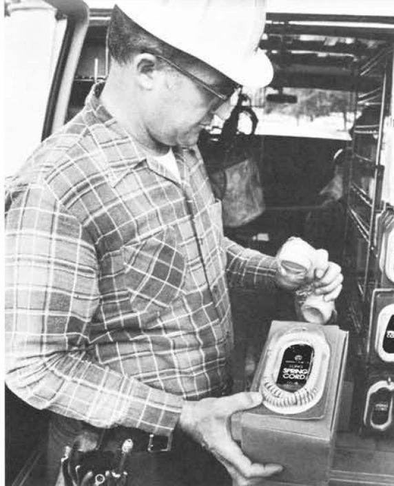
Service orders are a lot easier to fill with modular telephone sets. Robert Greenlee, installer-repairman for Illinois Bell's South Chicago district, selects parts from his truck inventory to assemble a modular set "to order" at the customer's home.
