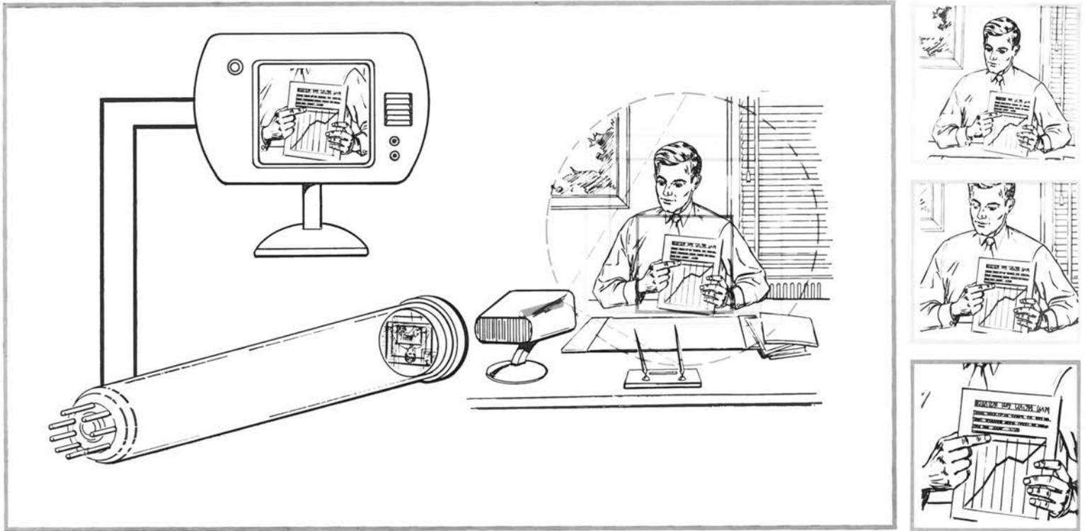
*The new camera tube electronically controls the field of view of the displayed image by changing the size and position of the scanned area on the target. The camera lens produces a fixed-size image. The displayed image is defined by the raster which can be varied by varying the beam accelerating voltage*
