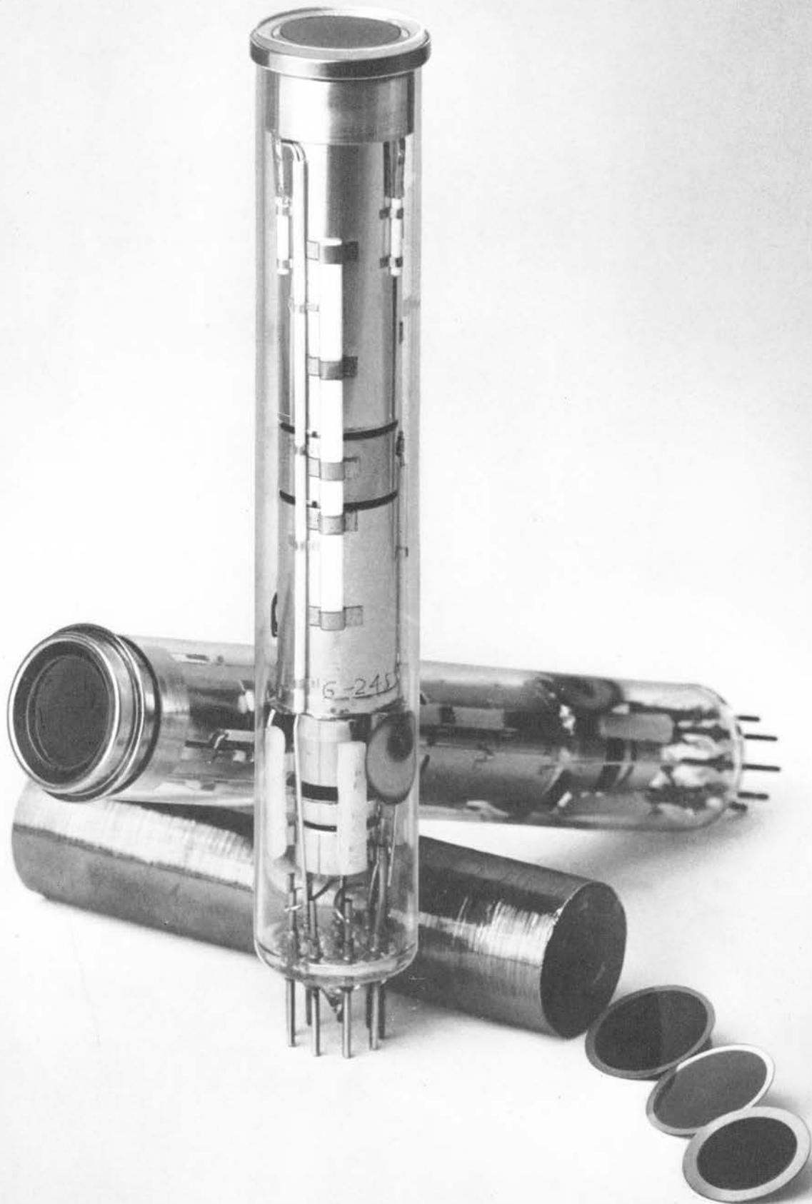
*A new camera tube for the PICTUREPHONE set uses an integrated silicon photo-diode array combined with conventional electron beam scanning. The result is a vidicon-type of camera tube which is far more sensitive and reliable than any now being used.*
