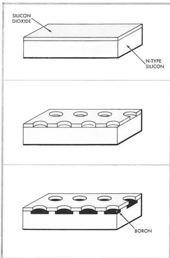
*Major processing steps (sequentially top to bottom) in the fabrication of the diode array. It starts as a silicon wafer several thousandths of an inch thick. An oxide layer about 25 millionths of an inch thick is then grown on the surface of the silicon. Photo-lithographic techniques are used to generate an array of holes in the oxide. Boron is diffused into the silicon through the holes forming the p-type islands. In this step the remaining oxide serves as a diffusion mask.*
