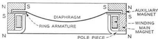
Fig. 3—Simplified view of ring armature receiver.
