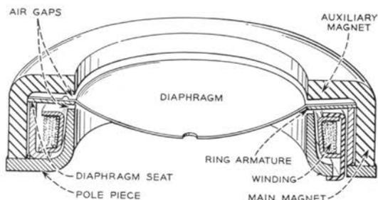
Fig. 2—Ring armature receiver.
