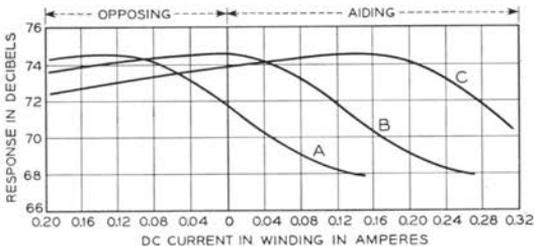
Fig. 4—U1 receiver response characteristics. A—Over-magnetized receiver. B—Correctly adjusted receiver. C—Under-magnetized receiver.
