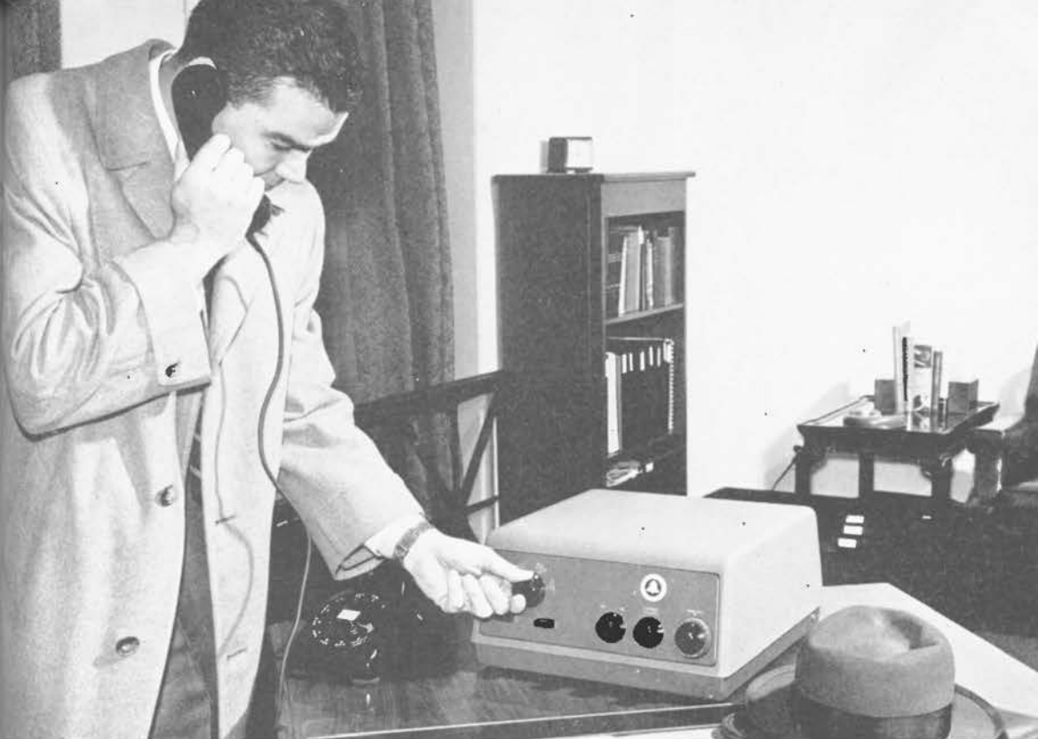
A customer records a statement on his automatic answering and recording equipment before leaving his office unattended. Upon his return he will listen to messages telephoned by people in his absence. Two types are available.
