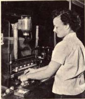
In this operation in the Company's Indianapolis plant, a machine is used to place carbon granules in the transmitter of the new "500" set. Hundreds of granules are needed to fill one assembly.
