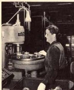
By means of this machine in the Indianapolis plant, the center post or bearing is pushed into the dial frame. The operation is performed by hydraulic pressure.
