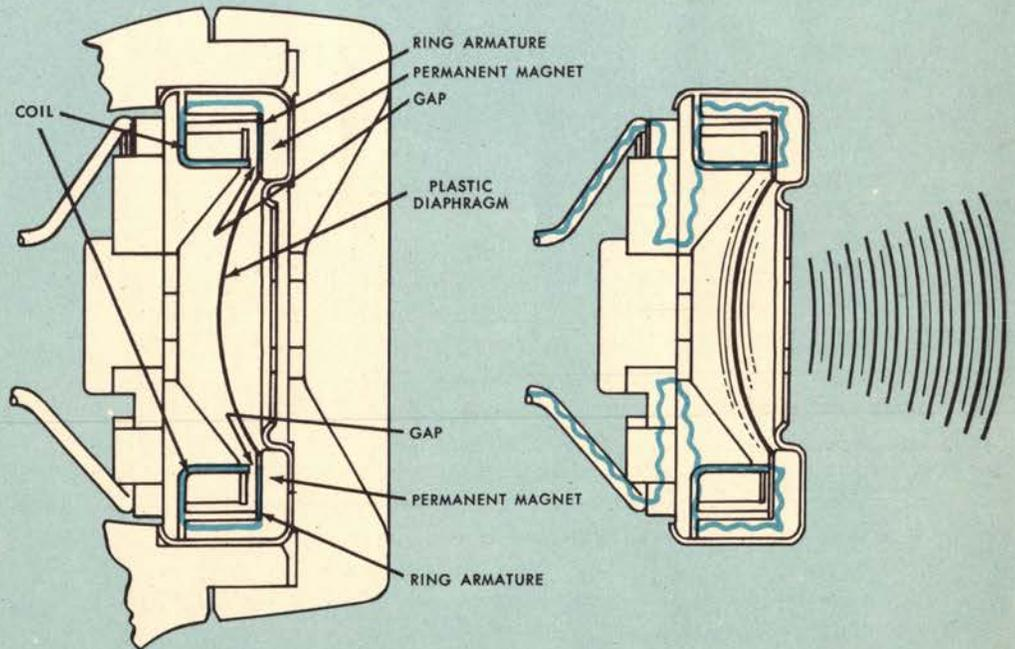
**B** With the parts assembled, but with no current reaching receiver, magnetism flows through as shown here—
