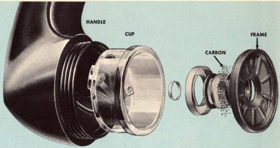
**A** Here are the parts of the transmitter
