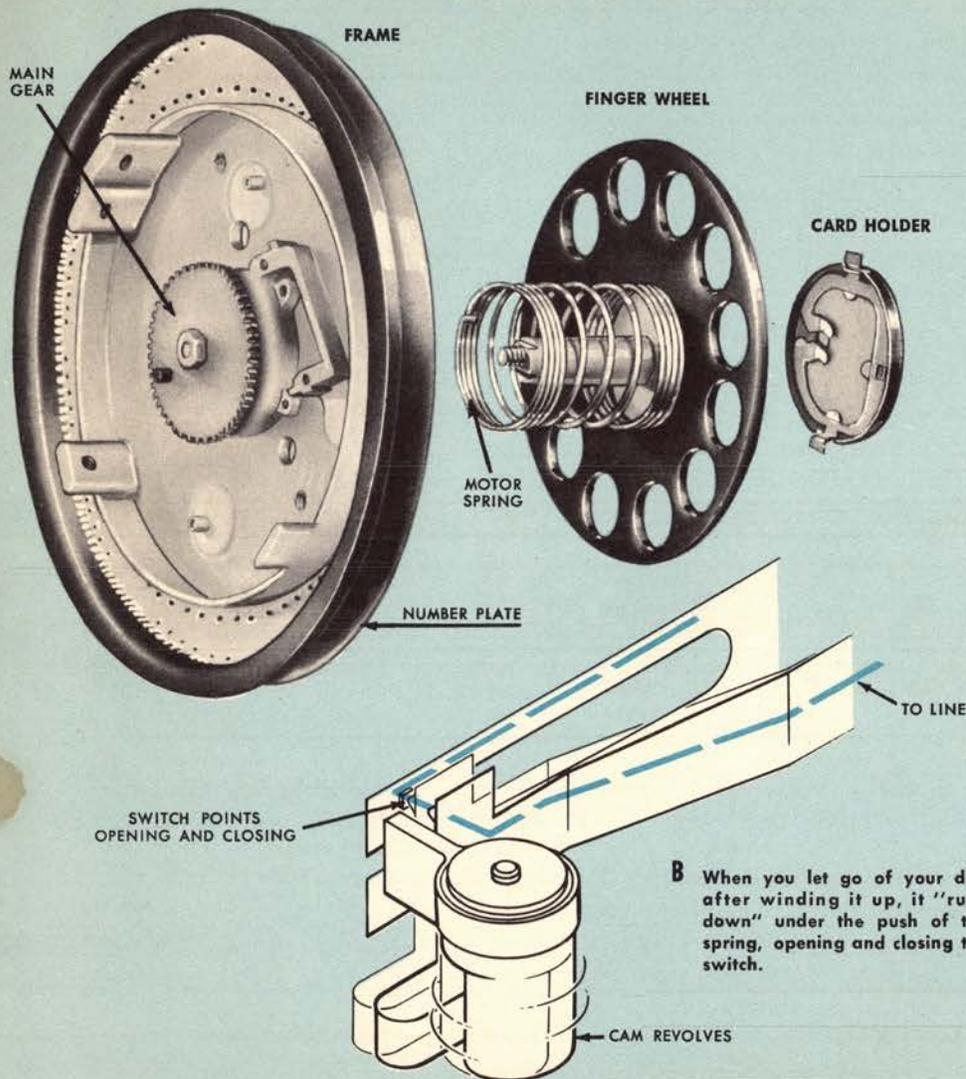
**B** When you let go of your dial after winding it up, it "runs down" under the push of the spring, opening and closing the switch.
