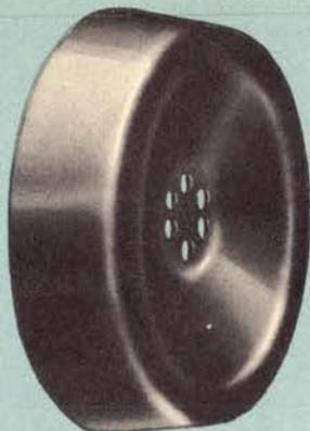
When the lines from two telephones are connected in the central office, the current flows into the receiver of the called telephone, and there sound is created for the listener. Pictured above are the receiver parts involved in this ingenious "trick."
