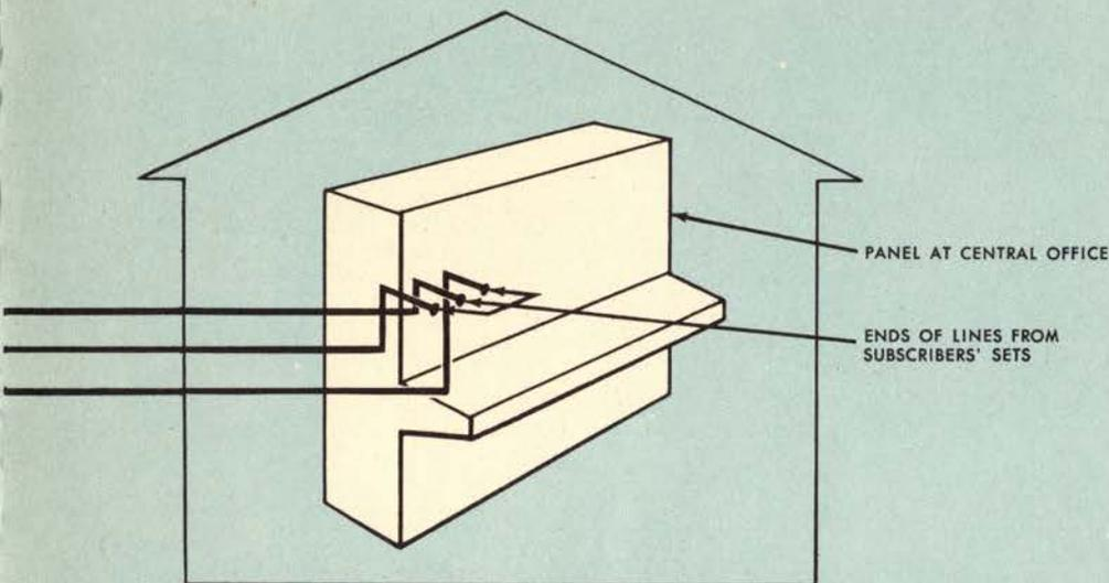
Now let's consider the operation of the central switching point shown in the simplified telephone system on Page 4. The lines from the three telephones are brought in to this point so that any two sets can be connected together for the duration of a conversation, and then disconnected.
