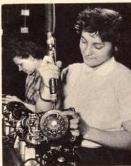
This operator is fastening the completed calling dial into position during final assembly operations on the "500" set.
