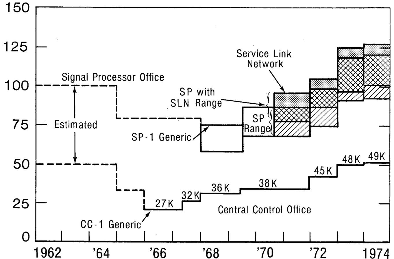
\* For signal processor offices the graph represents central control capacity as computed by ESSICAP. For generics SP - CTX - 5 (1972) and beyond, the signal processor may limit capacity in some offices. In these cases, office capacity will be less than shown.
