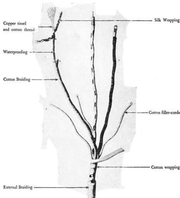
Each of the sets of copper ribbons carrying current is wound spirally around a cotton thread to make it spring-like and long lived. A cotton thread is used to help make round the group of conductors and over the grouped conductors is a braided cotton covering for insulation and protection on switchboard cords like this.
