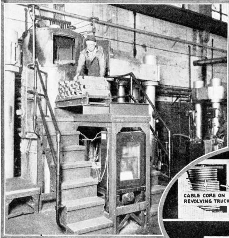
Left—Making lead sheathing to protect telephone wire starts with melting the pigs of lead for the lead press.
