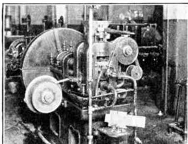
*This rolling mill is used to make the thin strips of duralumin from which is made the diaphragm in the transmitter of your telephone.*
