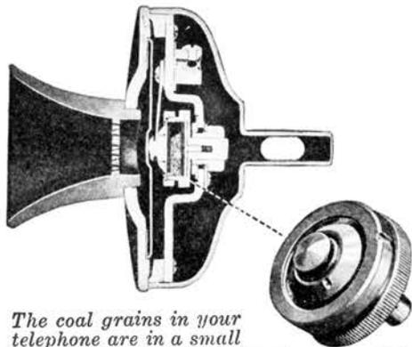
*The coal grains in your telephone are in a small receptacle just behind the aluminum diaphragm of the telephone transmitter.*
