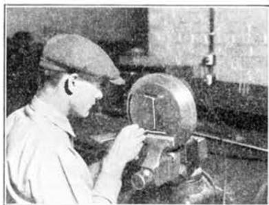
*A die through which aluminum is forced by a press to form an I-beam.*
