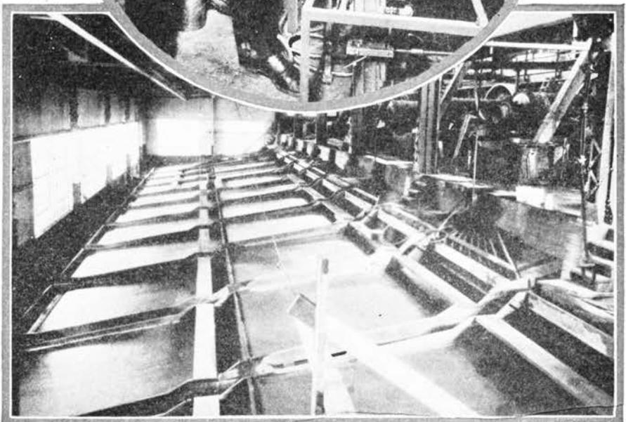
*When the amount of gold in an ore is small the concentration process is used to eliminate materials that contain no gold. Sometimes this is done by passing the finely crushed ore over plates covered with quicksilver which the gold or silver join and from which they are afterward separated by heat.*
