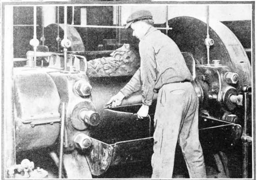
*Partially rolled sheets are slit and put through the rollers again and again to knead in the sulphur and other ingredients for vulcanizing the rubber.*
