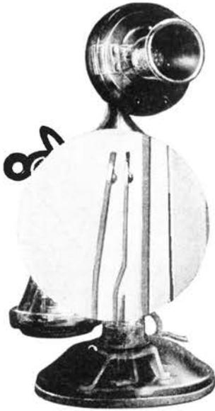
The two points on these upright springs are made from a gold, silver and platinum alloy. When you take the receiver off the hook, these springs come together until the points make contact—a path over which the voice currents travel.
