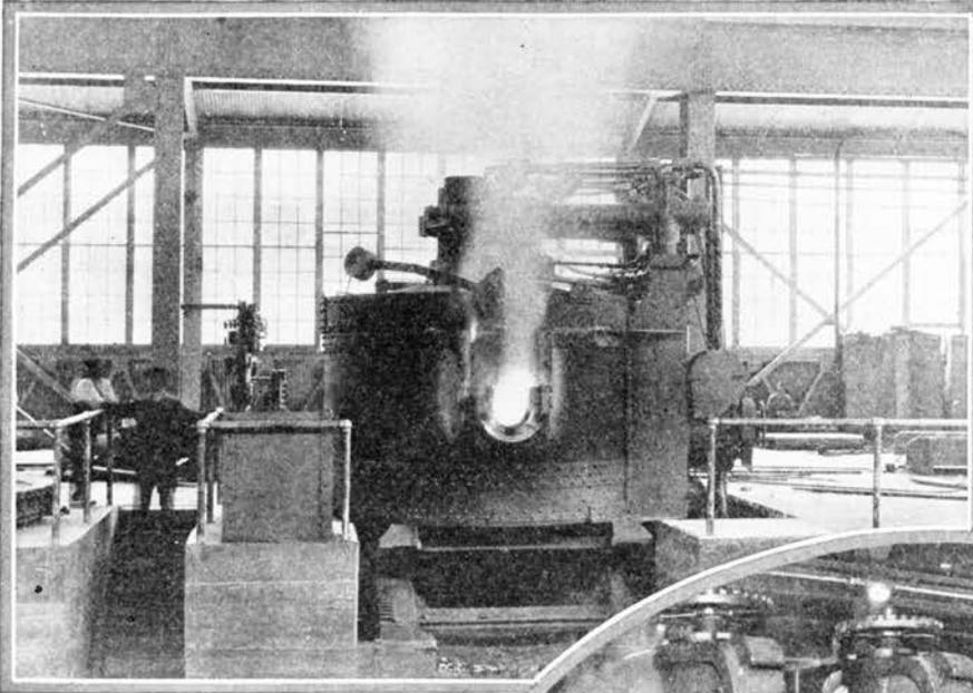
*Frequently, nickel is melted by electric heat. This electric furnace holds seven tons. The nickel is poured out of the nozzle from which the vapor is rising.*
