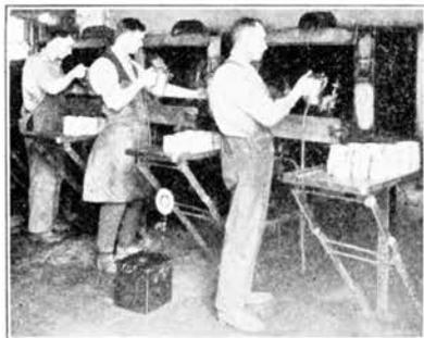
*The finish containing asphalt used on your telephone is sprayed on as if by an atomizer.*
