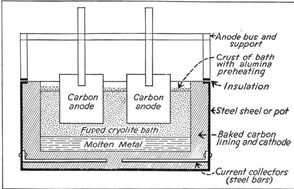
*Left—This sectional view of an aluminum furnace or "pot" shows the arrangement of the parts and materials described in the text.*
