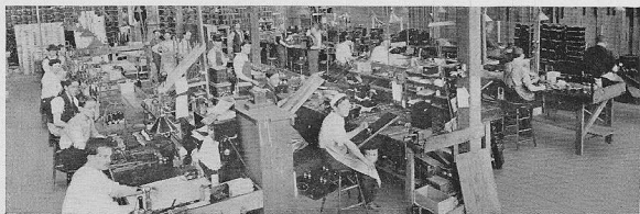
FIG. 62. — ADJUSTING RECEIVERS AND ASSEMBLING TELEPHONES. SECTION II
