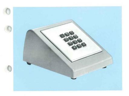
Stromberg-Carlson's 135 C3A TONE-DIAL pad allows you to give end-to-end signaling service even though the central office is only equipped for rotary-dial. It works this way: a computer access number, for example, is dialed in the usual manner on a rotary-dial telephone; once a circuit is established, the TONE-DIAL pad produces the tones required for information transfer. The pad can be used with a speaker-phone. Colors: page 13: white, beige, ivory, green, black, or gray.
