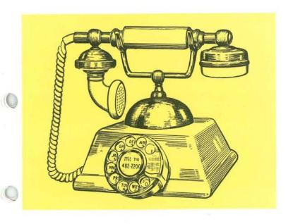
Everything is included to change that conversation piece into a working telephone. The kits are for decorator telephones which have been approved by the Bell System, and contain dial assembly, network, S-C P1A straightline ringer, transmitter and receiver capsules, cords, connectors, and hardware. The finger stop of our DE-209 is in a different position than the cut out in some decorator phones.
