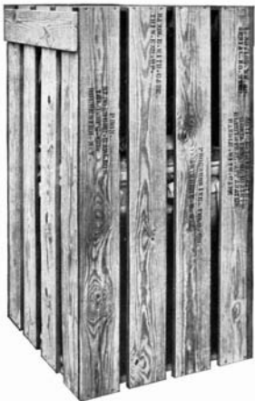
Fig. 29—Method of Crating No. 105 High Efficiency Switchboards for Domestic Shipment
