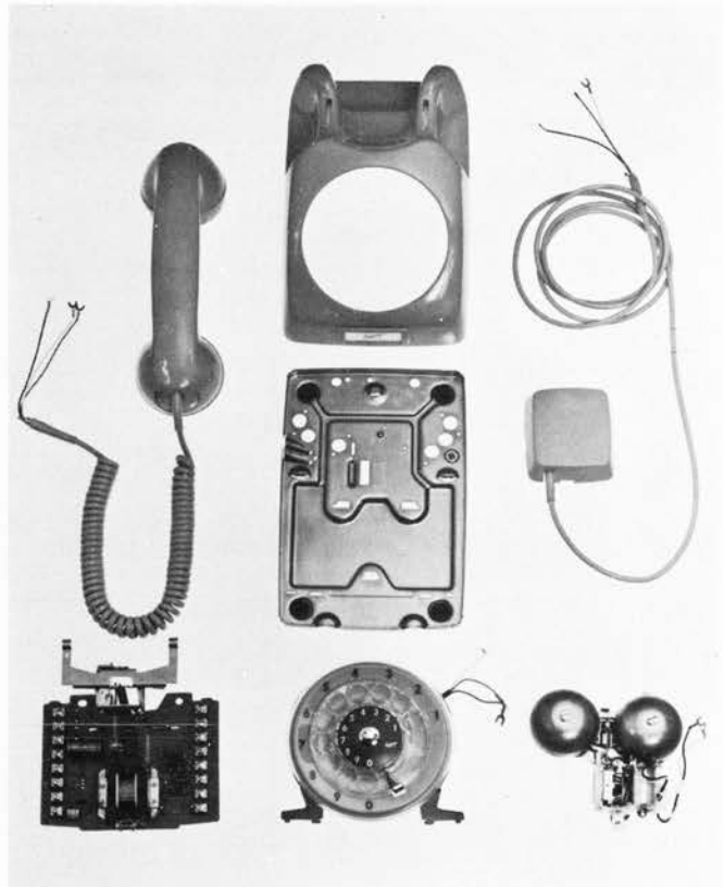
Fig. 4 The main parts of Dialog
