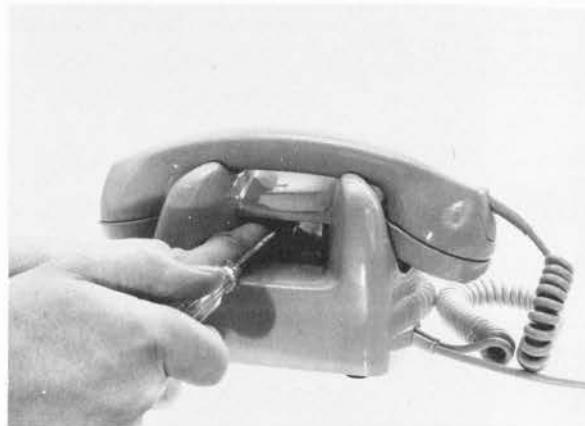
Fig. 6 The screw is well located for the repairman
