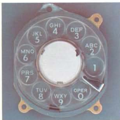
Type 10A —Miniature type with 2 \frac{3}{8} " numeral ring and automatic moveable finger stop. Designed for use in dial-in-handset telephones. Not provided with off-normal contacts.
