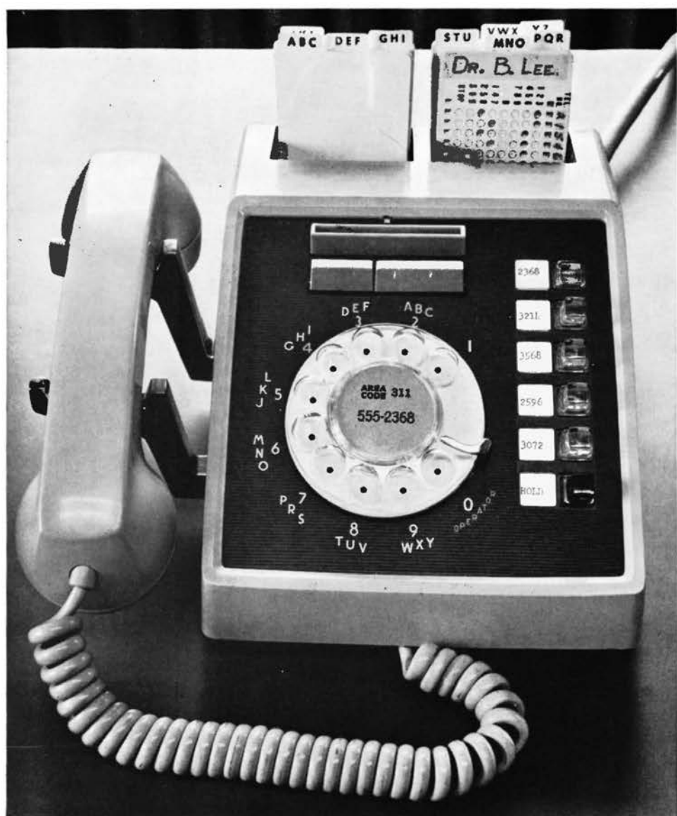
CARD DIALER telephone, a Bell System development, dials numbers precoded on plastic cards. It aids those who call the same numbers frequently, or numbers in specific sequences. Any number of cards can be prepared giving Card Dialer unlimited capacity.
