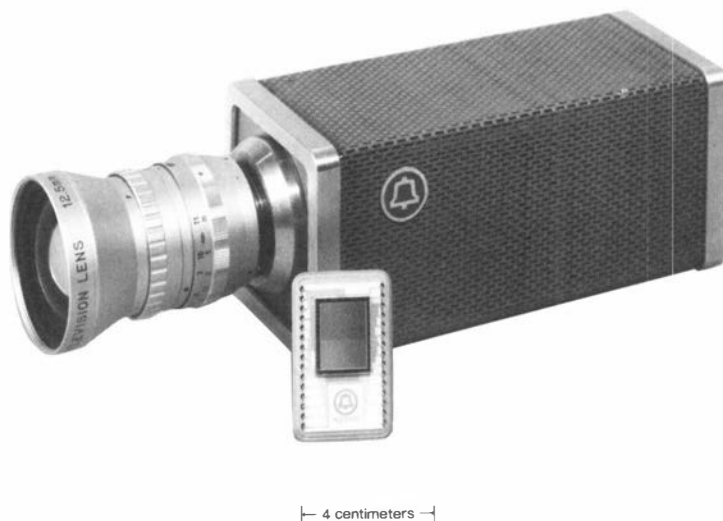
Fig. 4-10. Television camera with CCD imaging array. The CCD array consists of 500 by 500 picture elements.
