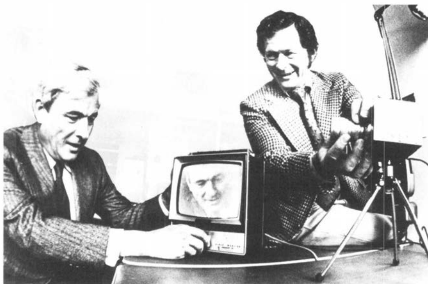
Fig. 2-15. W. S. Boyle (left) and G. E. Smith (right) demonstrating a TV camera using a CCD as a solid-state replacement for a conventional camera's vacuum tube.
