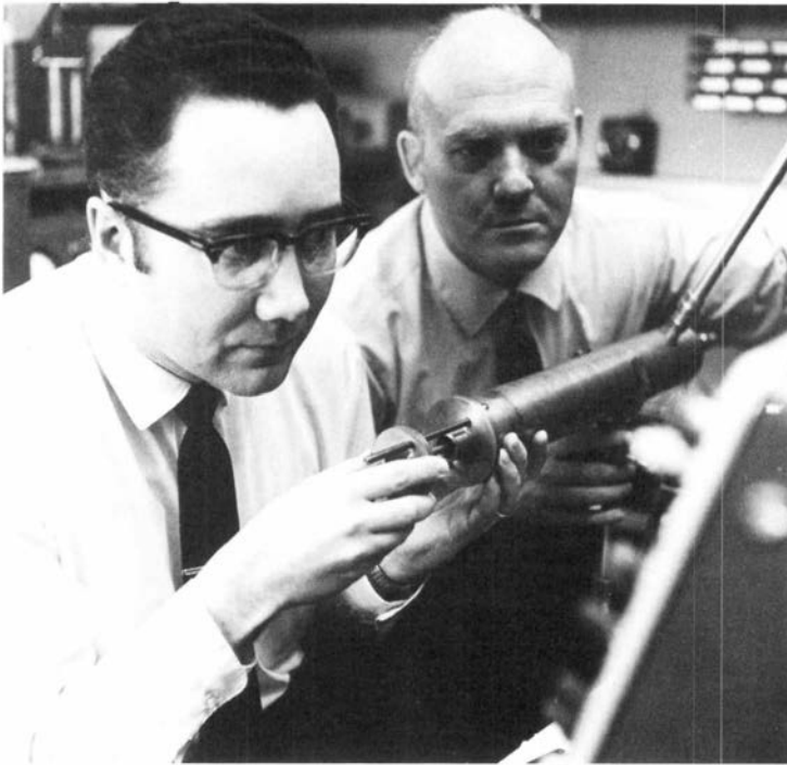
Fig. 1-43. B. C. De Loach (left) and R. L. Johnston (right) monitoring an oscilloscope while tuning microwave circuitry by moving the pistons in two intersecting brass tubes to optimize power output from an IMPATT diode.
