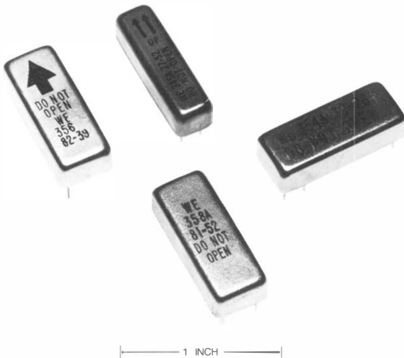
Fig. 7-11. Examples of the miniature mercury relay family. The 345-type and 356-type relays (marked with arrows) require fixed mounting orientation. The 354-type and 358-type relays can be mounted in any position.
