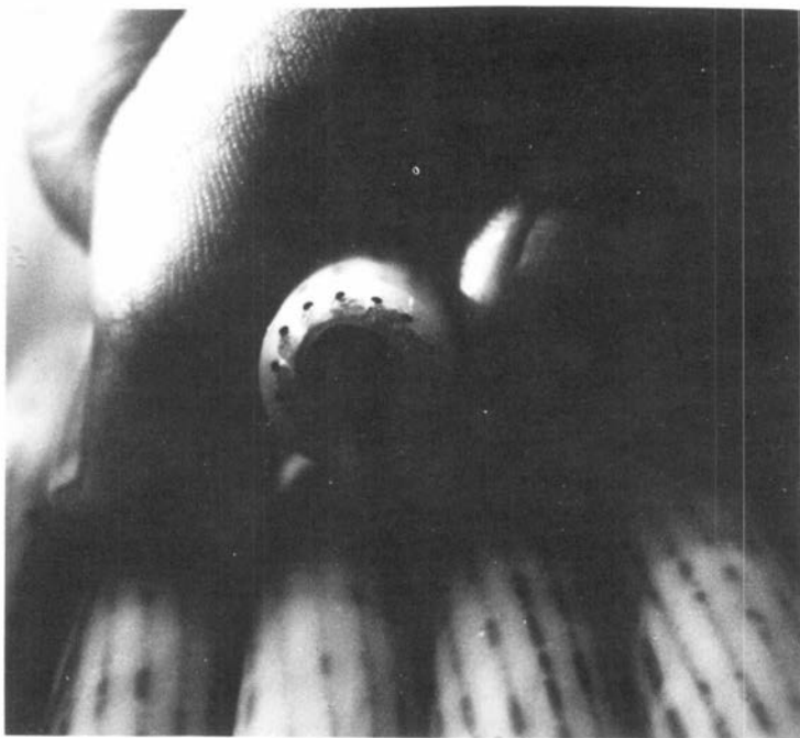
Fig. 4-16. Experimental fiberguide cable. Messages were transmitted via pulses of light in 144 fibers in the 1976 field trial in Atlanta, Georgia. [ Physics Today 29 (May 1976): cover.]
