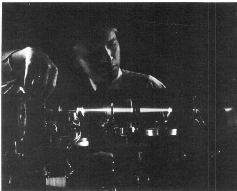
Fig. 4-2. S. Singh observing green light generated in barium sodium niobate from the invisible light output of an Nd:YAG laser.
