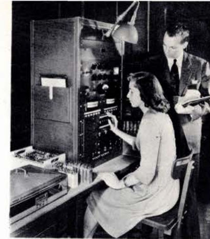
Testing one type of potted Thermistor. An airborne unit subject to rapid and extreme changes in temperature.
