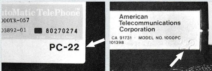
The Pocket Coder is designed to work only with the unit for which it was programmed. Check the number stamped on the metal plate on the end of the Pocket Coder and ensure that it matches the PC number stamped on the bottom of the base of The AutoMatic TelePhone.
