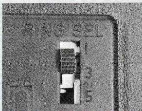
Some models have a three-position switch marked RING SEL on the bottom of the base. This switch may be set for one, three or five rings.
