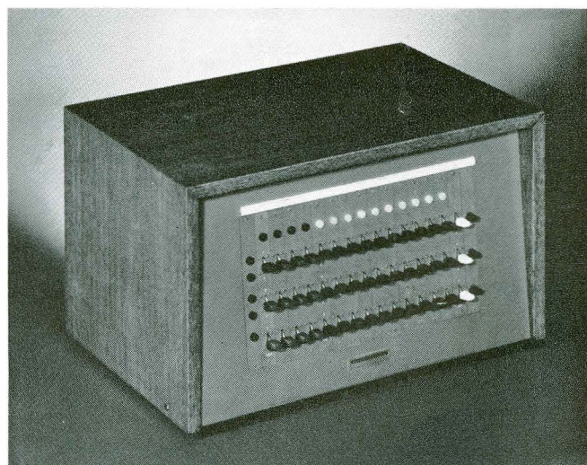
Cordless PBX—Two sizes: 10 lines, 4 trunks, 5 connecting circuits; 20 lines, 5 trunks, 5 connecting circuits. Can be supplied for 24- or 48-volt operation, and for use on automatic, manual, or magneto central-office trunks. A standard desk-type telephone is used as attendant's instrument. For full details, request Circular 1793.
