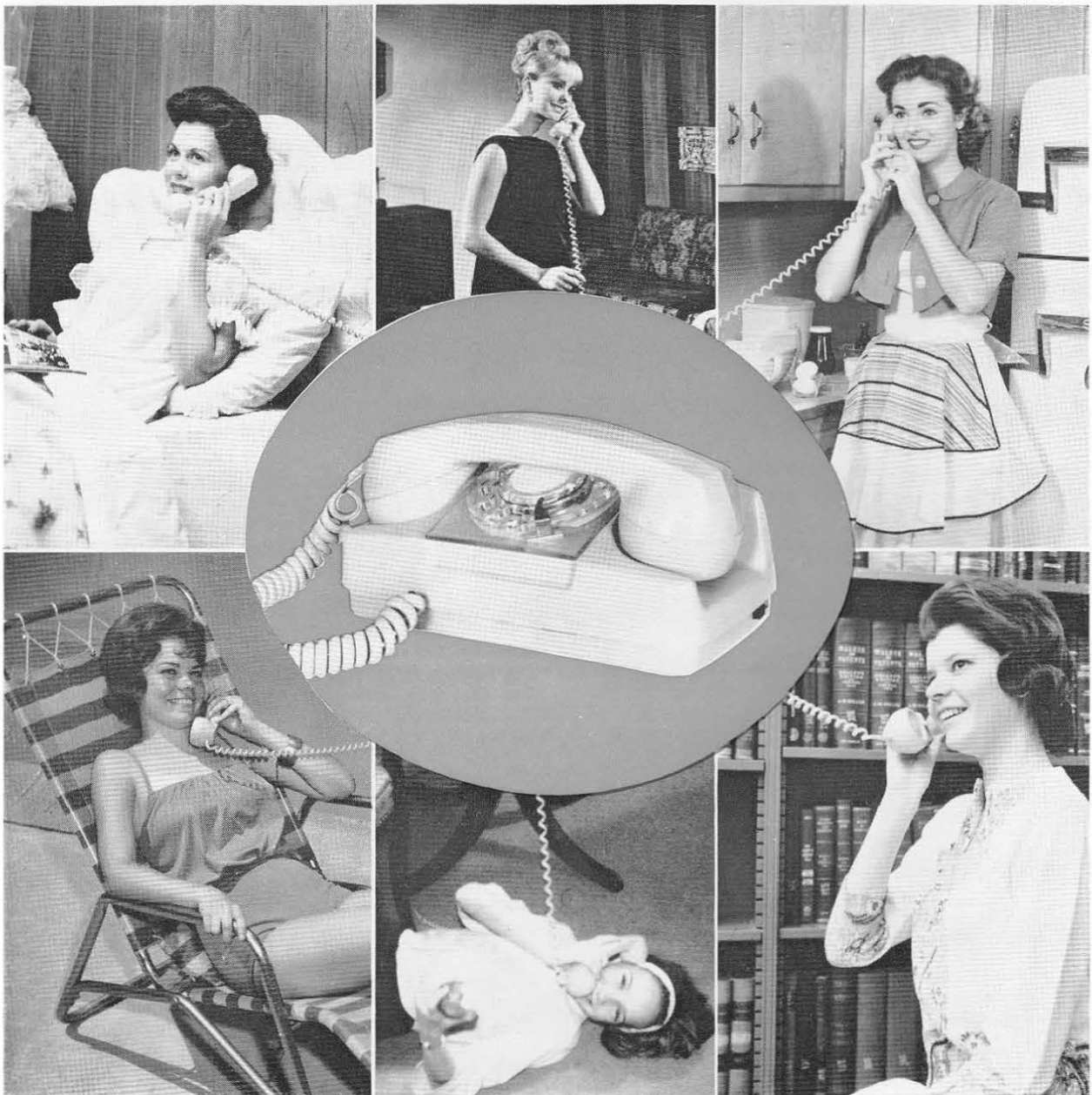
Figure 1. Starlite telephone with internal ringer can be used alone or as an extension in any part of the house or office. External appearance is unchanged except for dial-light control, which is located on the right rear corner instead of at the front-center of the base.
