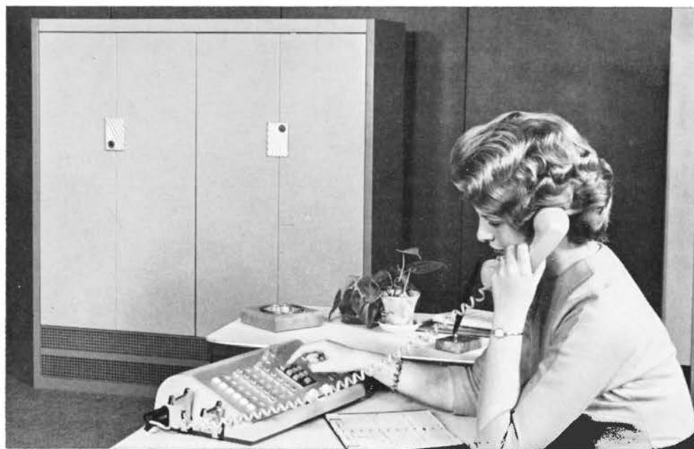
The attendant has a simple console from which calls can be completed with minimum attention from her. Cabinet in background holds switching unit, the only other equipment on customer's premises.
