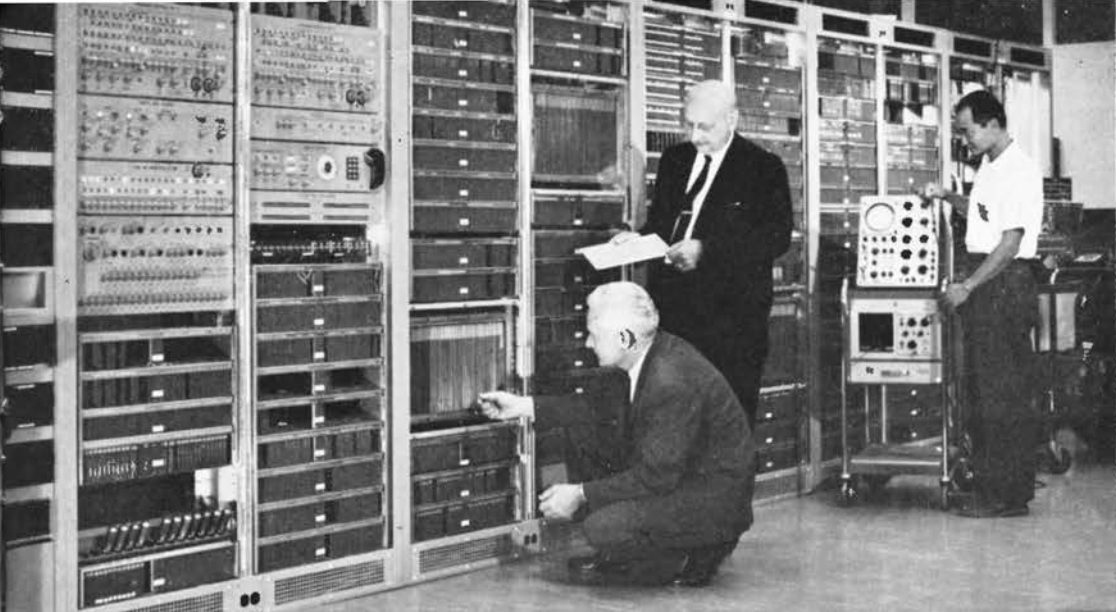
The 101 ESS control unit is located in the central office. It can serve as many as 32 businesses located within a radius of a few miles.
