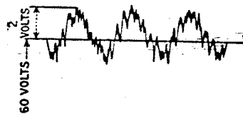
FIG. 194.—Voltage wave of typical commercial-type generator.
