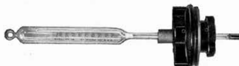
Vent Hole Thermometer with vent plug.
