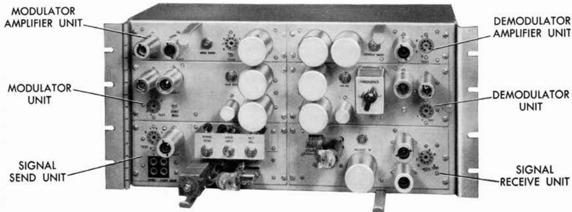
501 Carrier Terminal, front view, Cover removed
