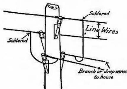
Fig. 40—Method of Attaching Branch or Drop Wires to the Pole.
