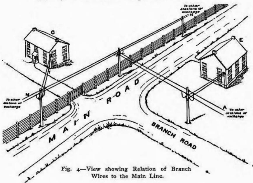
Fig. 4—View showing Relation of Branch Wires to the Main Line.
