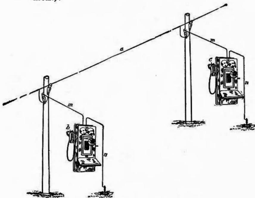
Fig. 1.—Diagram Showing Connections of the Grounded System.
